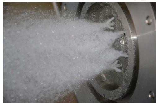
Figure 6: water test of the injecting plate.
